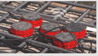
Figure 2. Embedded corrosion sensors
