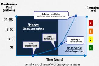
However, external environmental influences such as moisture and chlorides can cause internal damage that cannot be detected from the outside of the structure at early stages.
