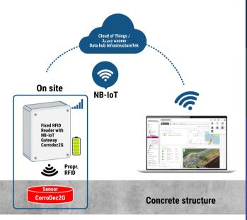
Our wireless sensors are passive and require no direct energy. It is power induced from the outside via a gateway or a handheld reader. Once the sensors are fully embedded within the concrete, it automatically transmits via our "Universal Monitoring System" to our Data Hub.
